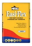
**PALACE EASI–FLEX** is standard setting polymer reinforced adhesive for fixing porcelain, vitrified & ceramic tile and stone to solid surfaces, heated sub-floors and Tile Backer boards. It offers the fixer a 4-hour working pot-life and allows grouting to proceed after 24 hours when it sets to a water-resistant bond suitable for interior / exterior use and in locations which are frequently wet or fully immersed.
