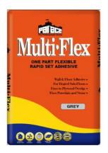
PALACE MULTI-FLEX is ideal for fixing all types of ceramic tile and stone to solid surfaces, heated sub-floors and Tile Backer boards. It is a fast setting grey or white adhesive and allows grouting to proceed 3 hours after it sets to a fully water-resistant high early strength bond suitable for interior / exterior use and locations which are frequently wet.
